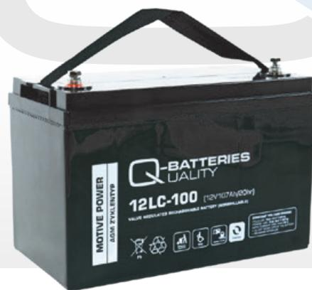
Q-Batteries Akku 12LC-100 battery is a special deep cycle battery which is designed for intensive cyclic discharge usage. Because of the very thick lead plates it's possible to achieve more cycles and longer lifetime. The 12LC-100 battery can be installed in any position except upside down.
