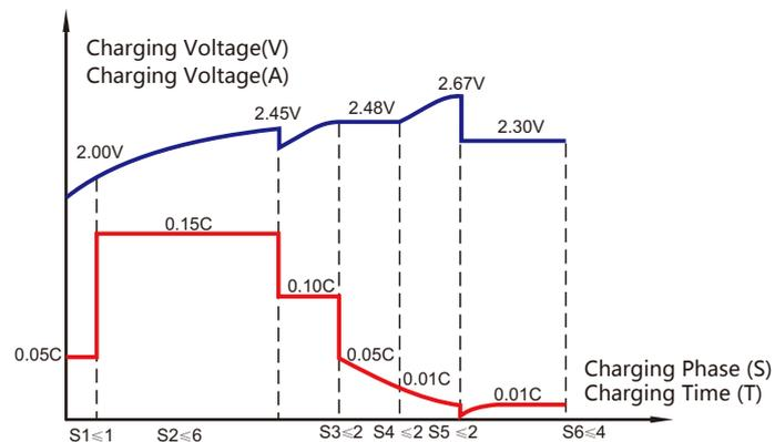
Note: The charging voltage values listed in the table are the voltages of a single battery at a standard temperature of 25 °C
